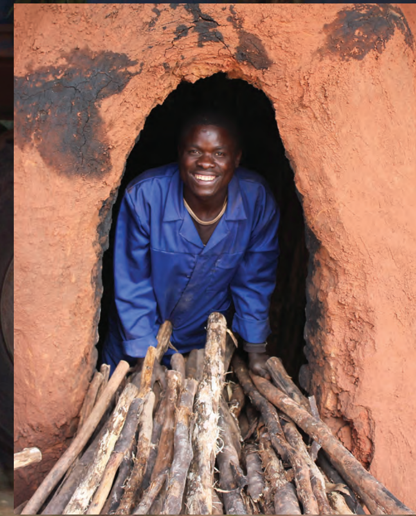
A KHP employee loads a half orange kiln with Corymbia citriodora offcuts to make sustainable charcoal © GINA ALTHOFF/TETRA TECH
